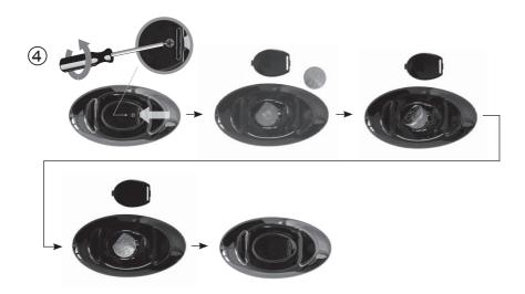
Before first use, loosen the screw (PH00 screwdriver), remove the back cover, remove the battery protection tab, replace the cover, retighten the screw.
